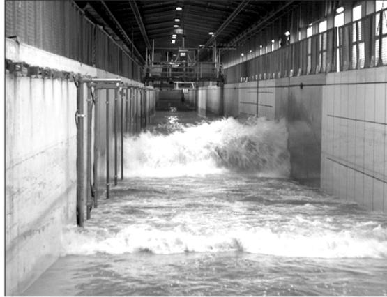
is about 900 kW. The gearwheel driven carrier gives a maximum stroke of  $\pm 2.10$  m to the wave paddle.
